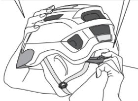
Hold the front side of the helmet and tighten the XF-8 Adjuster using the adjuster dial.
