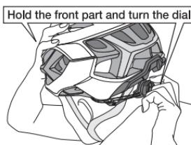
Holding the front side of the helmet and tighten the KBF-2 Adjuster using the adjuster dial.
