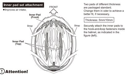
If air vents are covered by inner pads, air intake might be reduced. Attach inner pads correctly.
