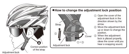
! Attention! Lock the cover securely after changing the position of the adjustment locks. If the helmet is used without locking the cover securely, the strap will be loose and the helmet may come off.
