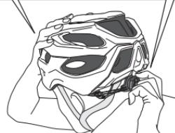
Holding the front side of the helmet and tighten the KBF-2 Adjuster using the adjuster dial.
