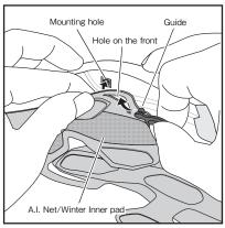
①Pass the adjuster guide on both through the A.I. Net/Winter Inner pad front holes. Insert the guide in the mounting holes.
