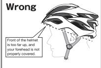
**OCAUTION** By wearing the helmet properly and fastening chin strap securely, it is possible to maximize the protecting functions of your helmet in the event of an accident. Therefore, wear your helmet properly before riding.
