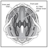
④On the hook-and-loop fasteners that outcropped from the holes of A.I. Net/Winter Inner pad, attach the top pad at the correct position.
