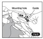
①Push the pins at the both guides into the mounting holes. (Upon using the A.I. net, put through the guide edge into the hole of the A.I. net then, attach the guide on the helmet.)
