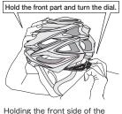
helmet and tighten the KBF-1 Adjuster using the adjuster dial.
