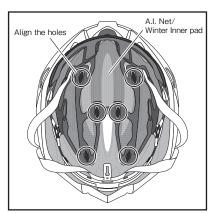
③Align the holes on the A.I. Net/Winter Inner pad and hook-and-loop fasteners on the helmet side to attach the A.I. Net/Winter Inner pad on the correct position.
