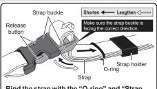
Bind the strap with the "O-ring" and "Strap holder" at the end.
